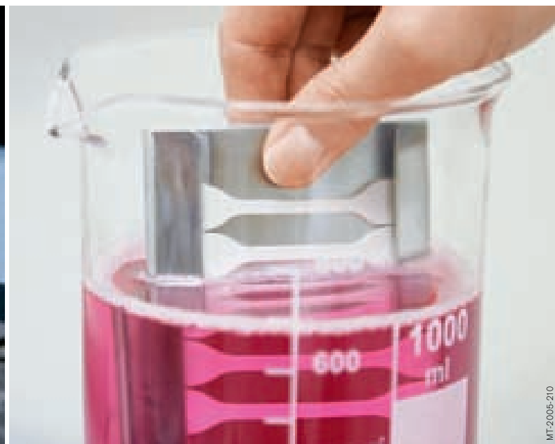
Testing pre-stressed plastic sample rods in cleaning fluid
