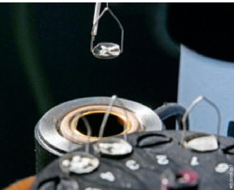
Sample prepared for thermogravimetry (see p. 29)
