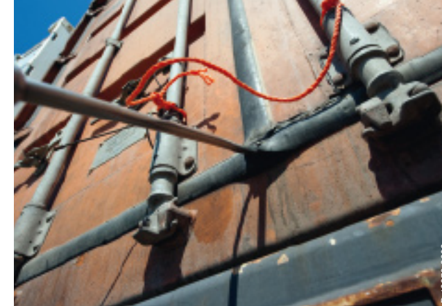
A journey of discovery with the probe: No one can say with certainty what gases are in the sealed container and will be released when the container is opened. Measurements provide certainty.
